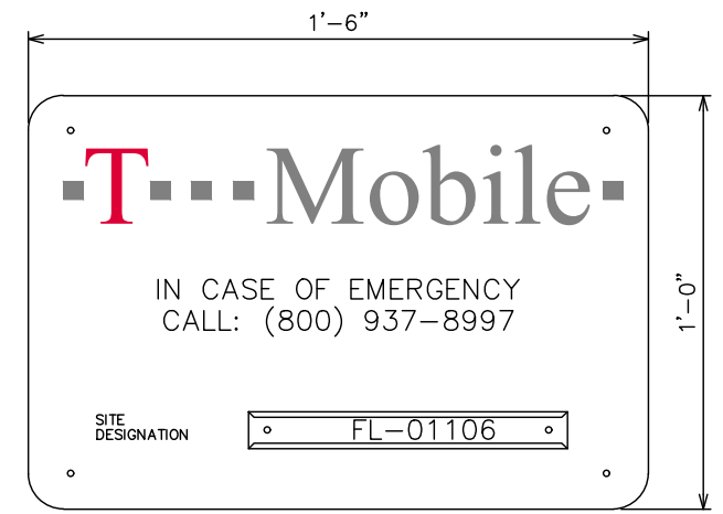
EMERGENCY SIGN (RED METAL W/ WHITE LETTERING)
