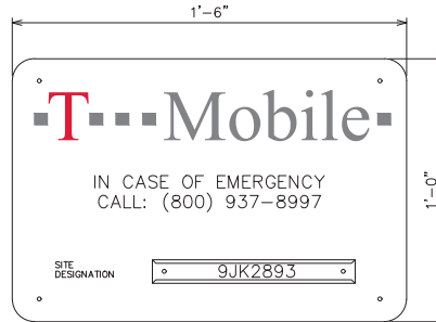
EMERGENCY SIGN (RED METAL W/ WHITE LETTERING)
