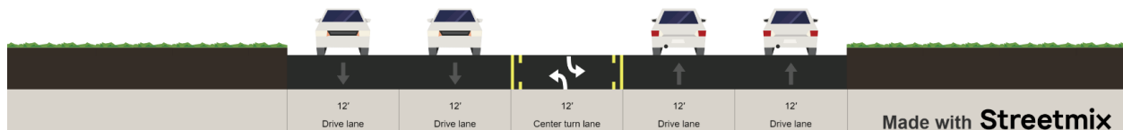
Figure 5. Maricamp Road — Existing Conditions — Typical Section
